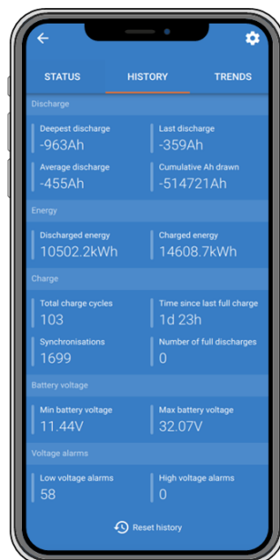
The VictronConnect app battery monitor history screen.
